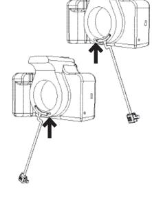
Attach camera lens to camera body.
