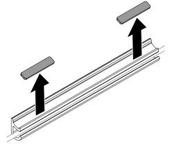
Remove the old adhesive from the underside of the trim piece.
