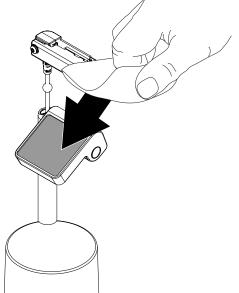
Peel one of the supplied square adhesives from it's backing and place on the bottom of the OEM charger and trim piece. Apply pressure for at least 10 seconds.
