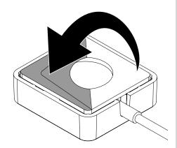
Place the OEM charger/cradle assembly onto the cradle. Make sure that the adhesive sits in the depression and press the trim piece, NOT the charger, against the cradle for at least 10 seconds.
