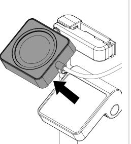
3 Remove the old adhesives from the cable guide.
