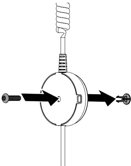
9 Use T20 bit to screw sensor to mounting plate using 1 provided screw.
