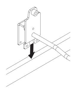
Install the the 2 screws to secure the hook bracket to the hang bar.
