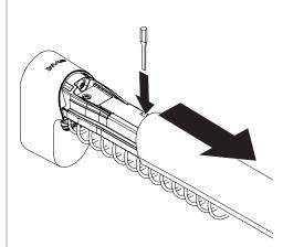
While holding the barrel open, feed the hook through the hole in the back of the rear housing. Ensure the hook feeds all the way through the coil.
