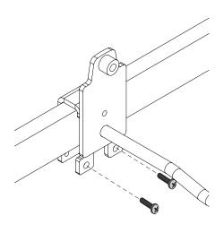
Hold the rear housing in one hand and slide the barrel several inches away from the rear housing. Hold the barrel in place. Note: Insert the sensor removal multitool attachment (AF6313) into the slot on the top of the T1000. If
