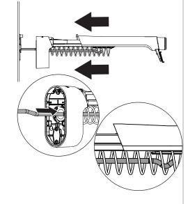
Push the T1000 against the wall while aligning the screw with the hole in the screw plate. Continue to hold the barrel open.
