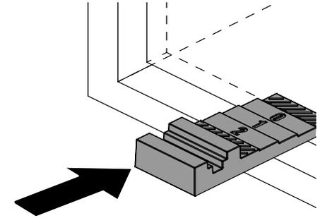
**3** Please consult the table below to determine how many (if any) shims need to be used, based on the number read in step 3. If either step with the diagonal lines fits between the edge of the door and the cabinet frame, do NOT install the L440.
