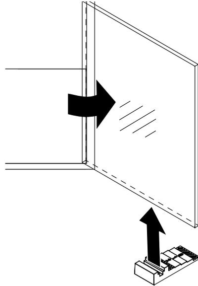
**1b** If the glass does not fit into the gauge or fits into the smallest groove do NOT install the L440.
