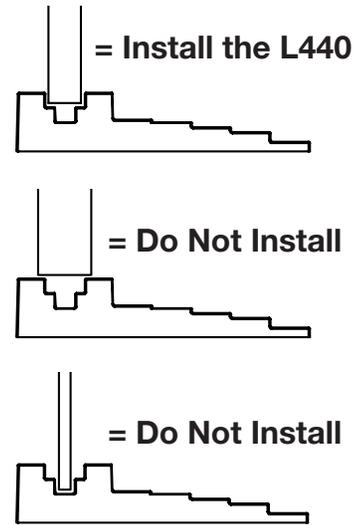
**2** Determine the gap between the edge of the door and the cabinet frame by inserting the sizing tool between the edge of the door and the fixture frame where the L440 will be mounted, as far as it will go without forcing it. Read the number on the step that fits between the edge of the door and the cabinet frame.
