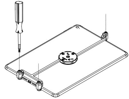
8 Use the mounting bracket screw to push the plug out from the sensor.
