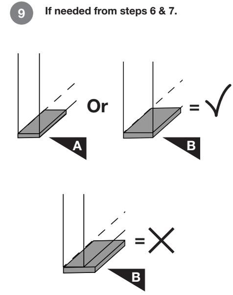
**CAUTION:** Be sure that the shim is not wider than the thickness of the glass door.
