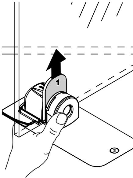
Note: Be sure that the lock housing is pressed firmly against the glass.
