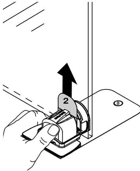
Note: Be sure that the lock housing is pressed firmly against the glass.
