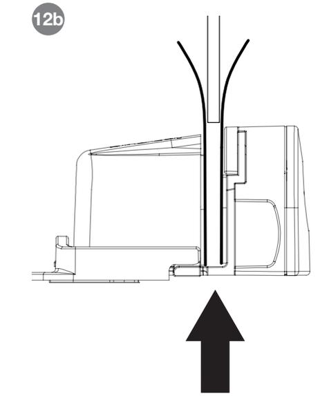
**CAUTION:** Be sure that the glass goes between the 2 adhesive liners on the lock housing and that the lock is pressed against the bottom edge of the glass or shim (if needed).
