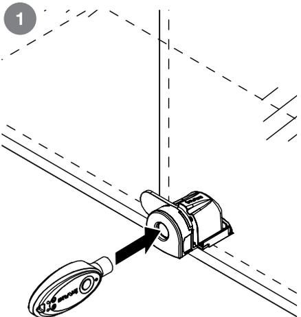
**Note:** If the key does not beep and makes a “knack-knack” sound it means the key was pulled away too soon. Try again and wait for the beep before pulling the key away.
