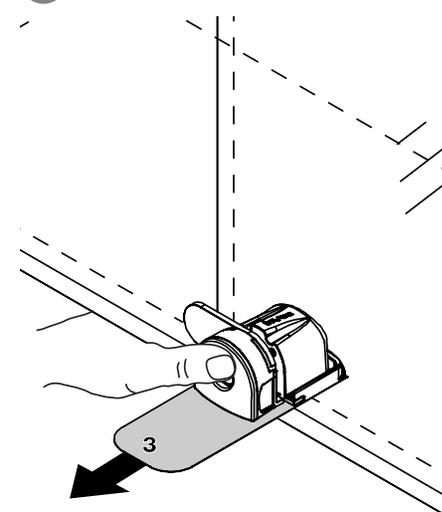
CAUTION: Hold the door in the closed position while pulling the #3 adhesive liner.
