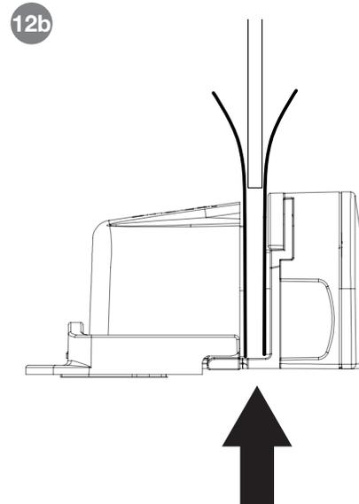
**CAUTION:** Be sure that the glass goes between the 2 adhesive liners on the lock housing and that the lock is pressed against the bottom edge of the glass or shim (if needed).
