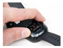
With the cable facing towards the top of the watch, place the sensor tray onto the watch body and apply pressure for at least 10 seconds.
