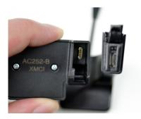
Align the micro USB plug on the charge head with the port on the stand.
