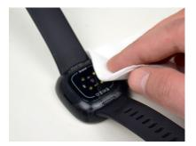
Use the provided alcohol wipe to clean the underside of the watch body.
