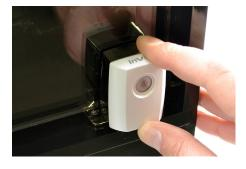
Press the lock body against the door panel for at least 10 seconds to seat the adhesives.
