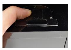
Apply pressure to the adhesive to hold the template in place.
