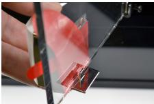
Slide the lock onto the door panel so that the door panel sits between the lock body and the tab on the base.
