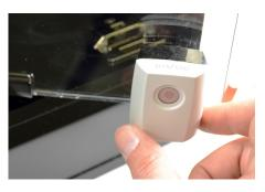
Open and close the door panel to ensure smooth interaction of the lock with the base plate.
