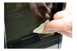
Use the provided alcohol wipe to clean the front of the door panel where the lock will sit. Allow it to dry completely.
