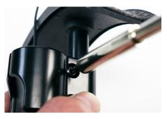
Use a TT20 bit to tighten the screw into the nut.
