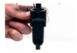
Close the brackets around the Cable Lock and headphone display post.
