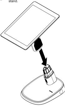
Plug the OEM power cable into the tablet and route the cable into the cable manager on the back of the base.
