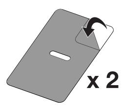
Center the 2 LSE plates, adhesive side down, onto the back of the device where the handle will be placed. Apply pressure for at least 10 seconds.
