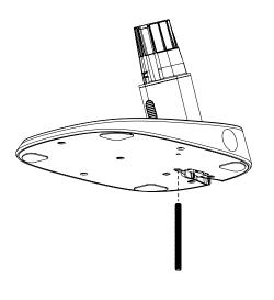
If drilling a hole for the stud mount, keep in mind that the stud is not centered in the stand. The stud will sit approximately 6 inches (5.94 inches, 150.8mm) from the front edge of the stand and 0.31 inches (7.8mm) from the center of the stand.
