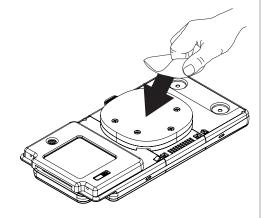
5a If using the Moby M120 version, remove the small rubber pad from the handle and insert the taller rubber stopper.
