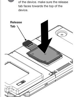
Place the dovetail plate onto the back
