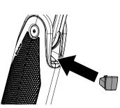
**5b** Orient the handle so that the arrow on the top will face the top of the device.
