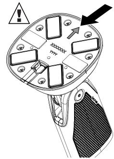
Remove the clear film from the adhesives on the CT80 handle.
