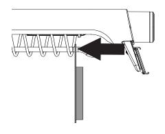
While holding the packaging against the coil, pull barrel to its full extension then return it to its closed position. Verify product is hanging on the rod and the coil is not threaded through the hangtab.
