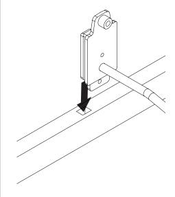
Install the screw to secure the mounting bracket to the hang bar.
