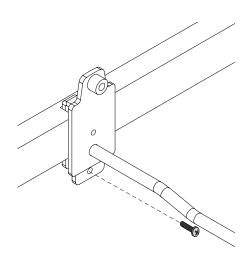
Hold the rear housing in one hand and slide the barrel several inches away from the rear housing.
