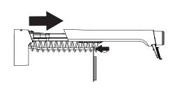
Repeat to load additional products, ensuring that one product is loaded in each coil space.
