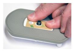
Smooth the adhesive onto the sensor cap for at least 10 seconds.
