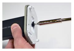
Use a TT15 bit to tighten the screw into the camera.
