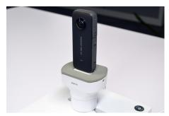
Place the sensor cap onto the sensor body.
