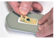
Align the large hole on the adhesive, sticky side down, with the screw on the sensor cap.
