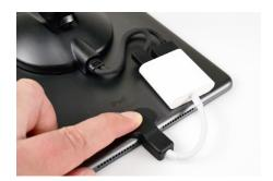
Place the procetive cap over the power connector, with the adhesives on the back of the tablet. Apply pressure for at least 10 seconds.
