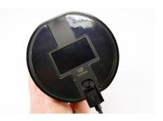
Peel the old adhesives and replace with new adhesives from the CT1509 replacement adhesive kit. The handle is now ready to be reinstalled.
