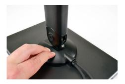
Center the handle on the back of the tablet and apply pressure for at least 10 seconds.
