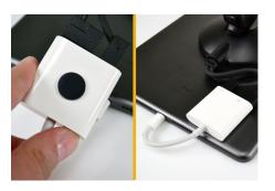
Optional: A small piece of adhesive can be placed on the adapter to keep it secured to the back of the tablet.
