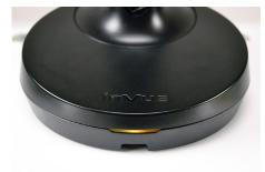
If the base is powered up before a handle is docked, the LED on the front will be orange.
