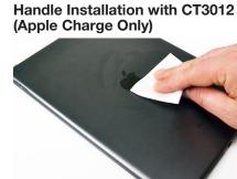
Use an alcohol wipe to clean the back of the tablet. Allow it to dry completely.
