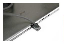
38 Plug the connector into the tablet.
