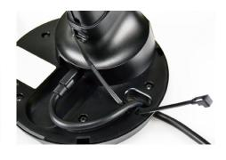
If installing a peripheral cable, lift the top cover from the base using the small lip above the LED on the front of the base.
