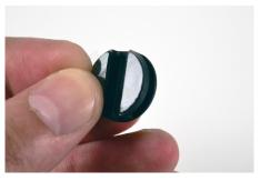
Peel the clear film from the 2 adhesives on the cable manager.
