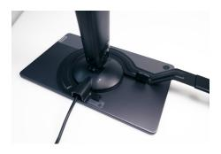
Place the CT1507 removal tool around the handle where it is adhered to the tablet.
