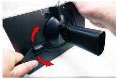
Place the tablet on it's side and apply force up and down to break the adhesive bond.
