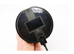
Plug the CT3012 power connector into the CT1503 handle.
