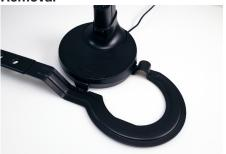
If removing the base, remove the handle and tablet from the base first. Then insert the hook of the CT1507 removal tool into one of the cable openings on the base. The padded tab should sit against the base.
