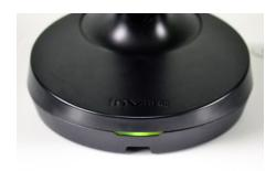
Once a handle is placed on the base, the LED will turn green to indicate that the tablet is recieving power.
