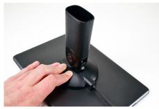
37 Center the handle on the back of the tablet and apply pressure for at least 10 seconds.
