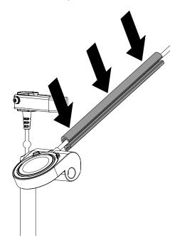
Peel the clear film from the 2 adhesives from the cable guide.
