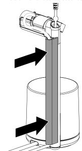
Ensure that the trim piece is installed in line with the back of the stem as shown.
