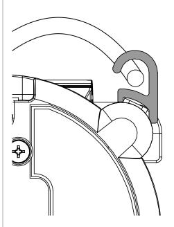
Route the cable along the track in the back of the cradle. Adjust the cable in the cable guide as necessary.
