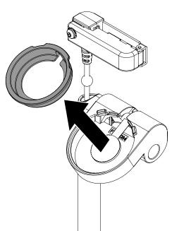
Insert the OEM charger cable through the center of the cradle insert.
