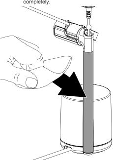
Route the OEM charger cable into the cable guide.
