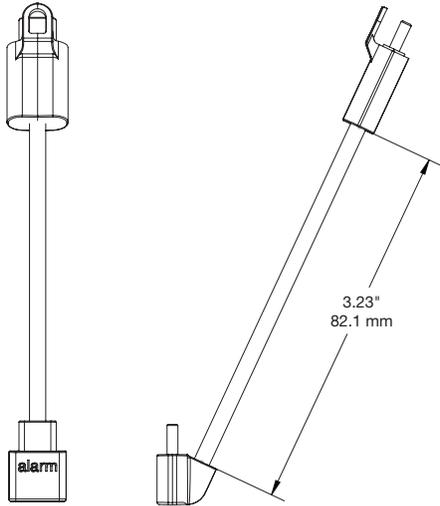
One55/One65/One60 Tablet USB Type C Power Connector (DBT501):
