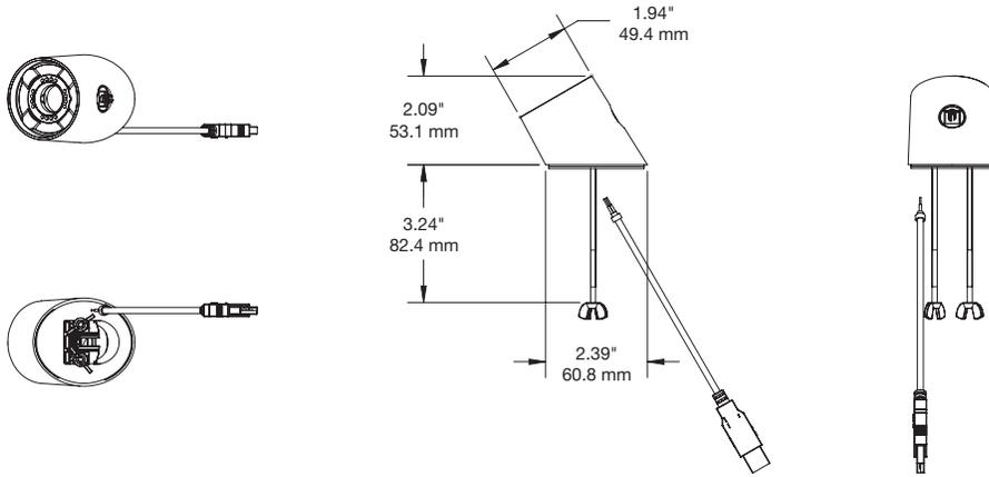
OnePOD Non Connected Recoiler Standard Cable (DBD300):
