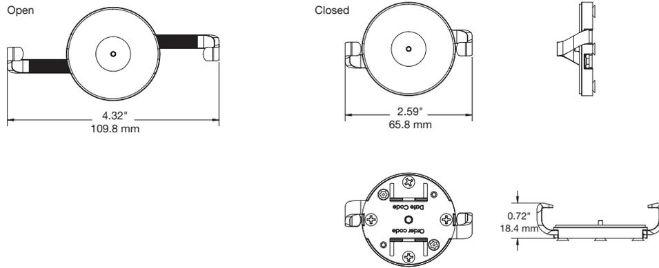
One55/One65/One60 2 Arm Bracket Plate with tablet brackets (DBT282):
