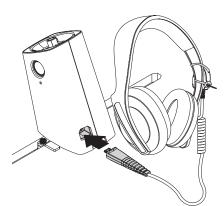
**Note:** Powered applications for auxiliary port are limited to a maximum 5V, 500mA.
