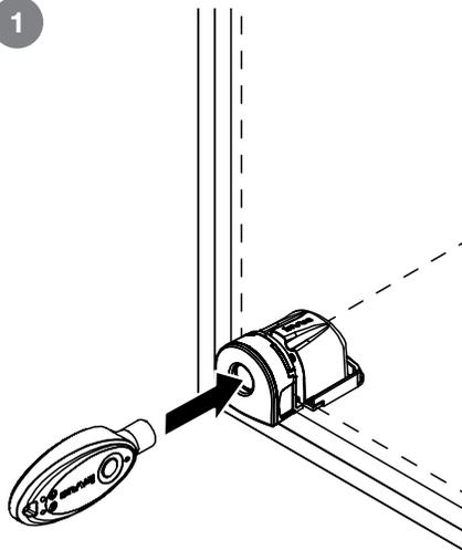
**Note:** If the key does not beep and makes a “knack-knack” sound it means the key was pulled away too soon. Try again and wait for the beep before pulling the key away.
