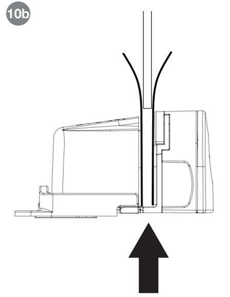
**CAUTION:** Be sure that the glass goes between the 2 adhesive liners on the lock housing and that the lock is pressed against the bottom edge of the glass or shim (if needed).
