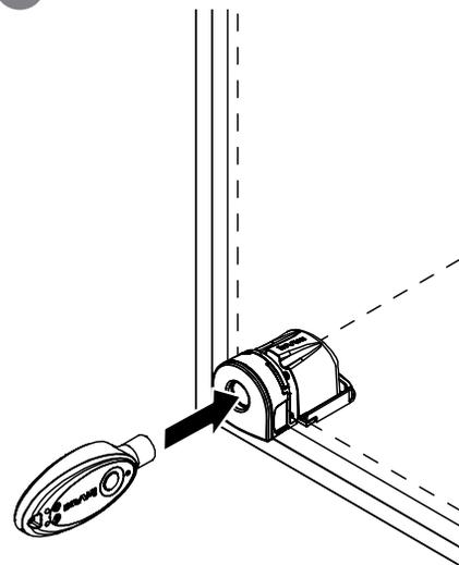
**Note:** If the key does not beep and makes a "knack-knack" sound it means the key was pulled away too soon. Try again and wait for the beep before pulling the key away.
