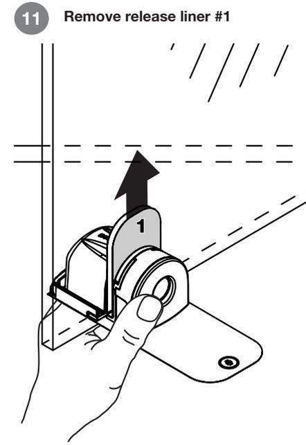
**Note:** Be sure that the lock housing is pressed firmly against the glass.
