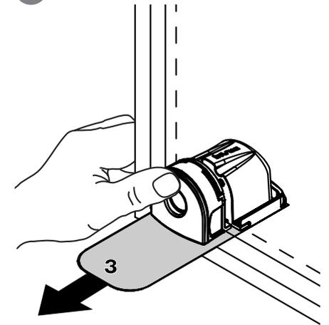
**CAUTION:** Hold the door in the closed position while pulling the #3 adhesive liner.
