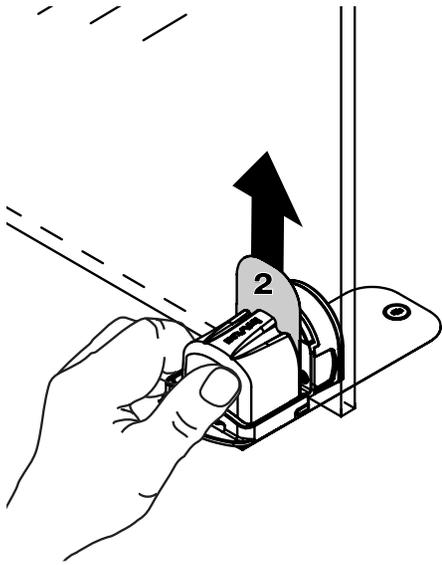
**Note:** Be sure that the lock housing is pressed firmly against the glass.
