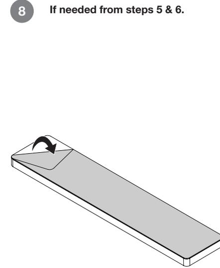
**CAUTION:** Be sure that the shim is not wider than the thickness of the glass door.
