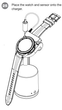
Plug the OEM charger cable into the power supply. Plug the power supply into an outlet. Make sure that the watch is receiving power.
