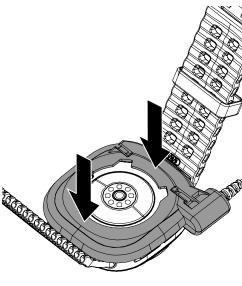
Lift the connector from the stand, pulling enough cable to aid in the installation of the sensor. Snap the included cable stop clip around the cable to prevent it from retracting.
