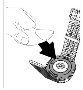
Press the band release button on the device and remove the buckle band.
