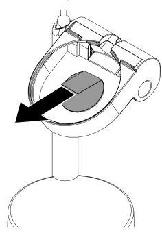
With the charger cable facing towards the groove in the charger cradle, place the OEM charger and cradle insert into the cradle. Apply pressure for at least 10 seconds.
