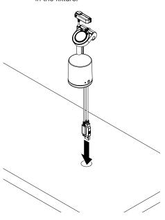
Place the stand in the desired location and apply pressure for at least 10 seconds.
