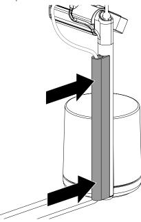
Route the cable along the track in the back of the cradle. Adjust the cable in the cable guide as necessary.
