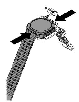
Press the watch body and tray sensor together for at least 10 seconds.
