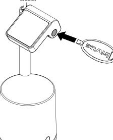
Remove the plug and use the TT8 bit to remove the screw from the side of the cradle
