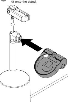
Secure the new cradle with the screw. Insert the plug into the hole in the side on the cradle.
