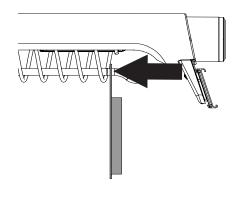
While holding the packaging against the coil, pull barrel to its **full extension** then return it to its closed position. Verify product is hanging on the rod and the coil is not threaded through the hangtab.
