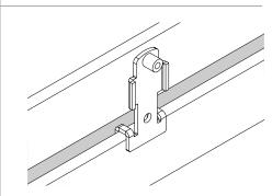
Hold the screw plate in place and install the hook plate into the slat wall groove with the prongs facing up.
