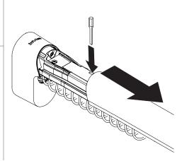
While holding the barrel open, feed the hook through the hole in the back of the rear housing. Ensure the hook feeds all the way through the coil.
