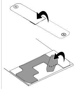
Attach the adhesive to the strike plate as shown and apply pressure for at least 10 seconds.
