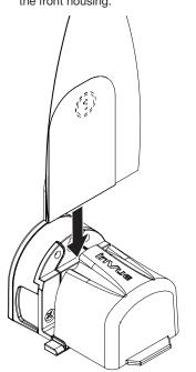
Use the putty knife to press the adhesive against the front housing for at least 10 seconds.
