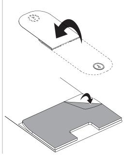
Attach the front housing adhesive to the front housing.
