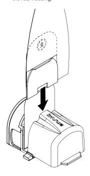
Use the putty knife to press the adhesive against the rear housing for at least 10 seconds.
