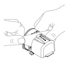
Fold the adhesive pull tab (labeled "1") for the front housing adhesive as shown. Remove the adhesive liner.
