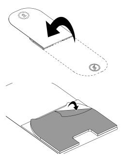
9 Attach the rear housing adhesive to the rear housing.
