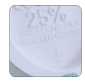
POST-CONSUMER RPS (POST-CONSUMER RECYCLED POLYSTYRENE) Polystyrene (PS) is a common petroleumbased plastic that can be identified using resin code #6. Just as with rPET, we use the highest amount of rPS that we possibly can in the different products we make from this material.
