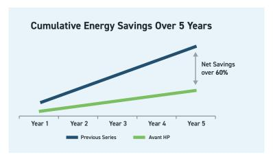
In the comparison scenario below, our new product line, Avant only required 37.5% of lamps or power consumption compared to the old product line (SCD-H). Avant met the same performance level to reduce TOC levels below 2 ppb with significantly lower power consumption.
