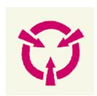
These industry standard ESD symbols are printed on the packing material to notify distributors and users that ESD precautions and proper handling procedures must be utilized to insure the reliability and quality of both the IC's inside as well as the electronic end products that will utilize them.
