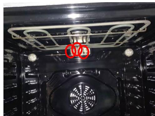
Be sure to reconnect the wires in the correct order/location for proper operation.
