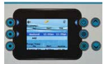
You can modify the schedules by selecting (middle left) lit button and adjusting the schedule using the or buttons. Press (middle left) lit button to move between parameters.
