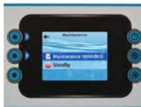
Once Standby mode has been activated a screen will appear to show that pumps are stopped. The normal fitness system page will return at the end of maintenance.
