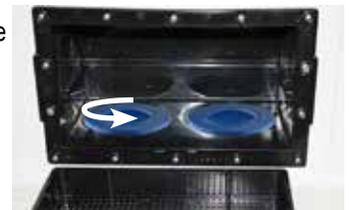
6. Pull filter up, then angle the top away from the filter compartment to pull filter completely out. Each filter has 50 sq. feet of effective filter area.
