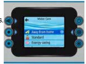
When in Economy mode, the heating set point will be reduced by 11°C (20°F), which means that the heating system will not come on during the set time unless the temperature falls 11°C (20°F) below the fitness system's set temperature.
