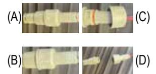
Disconnect Light bar wires (see steps A-D above)
