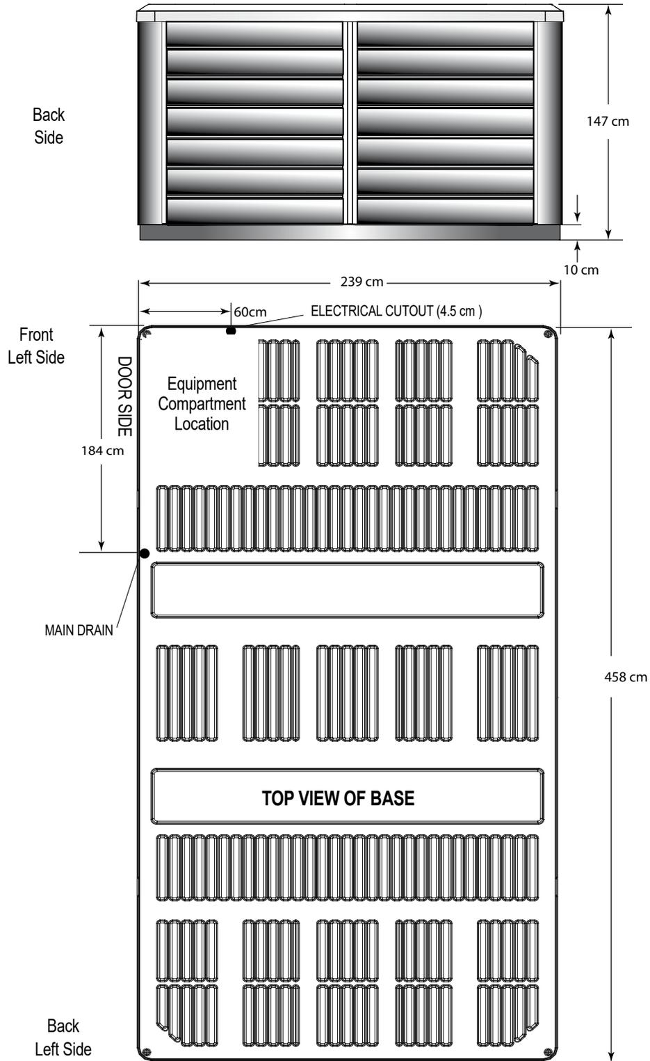
**NOTE: ENDLESS POOLS** requires that the E550 Models be installed on a minimum 15 cm (6") thick reinforced concrete pad or structurally sound deck able to support the "dead weight" found in the specification chart on the back page.
