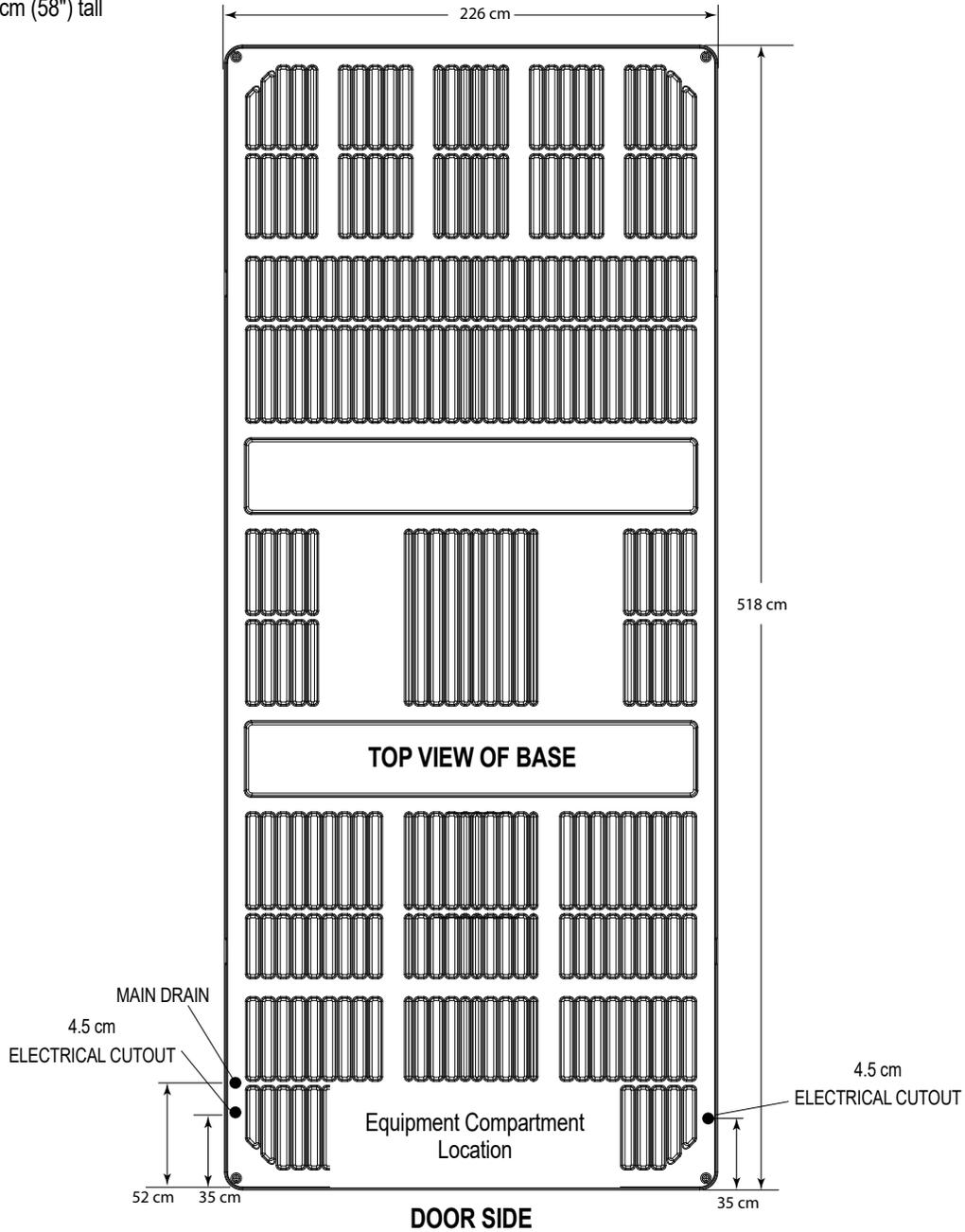
**NOTE: ENDLESS POOLS** requires that the E700 Models be installed on a minimum 15 cm (6") thick reinforced concrete pad or structurally sound deck able to support the "dead weight" found in the specification chart on the back page.
