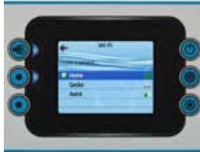
Once the in.touch 2 module is connected to a Wi-Fi network a green check mark will appear in the Wi-Fi menu, and the network name will appear in the Settings menu.
