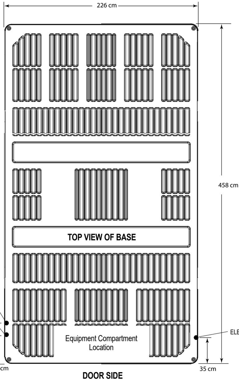
**NOTE: ENDLESS POOLS** requires that the E500 Models be installed on a minimum 15 cm (6") thick reinforced concrete pad or structurally sound deck able to support the "dead weight" found in the specification chart on the back page.
