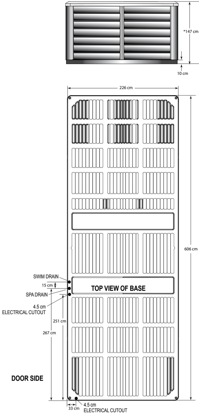
**NOTE:** ENDLESS POOLS requires that the E2000 Model be installed on a minimum 15 cm (6") thick reinforced concrete pad or structurally sound deck able to support the "dead weight" found in the specification chart on the back page.
