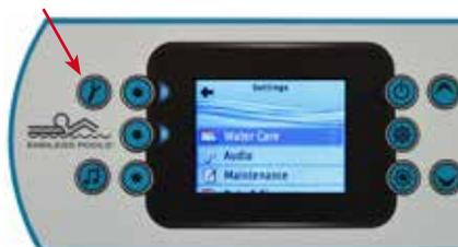
Use the or buttons to move up and down in the list. To select an option, press the lit button beside the desired highlighted option.
