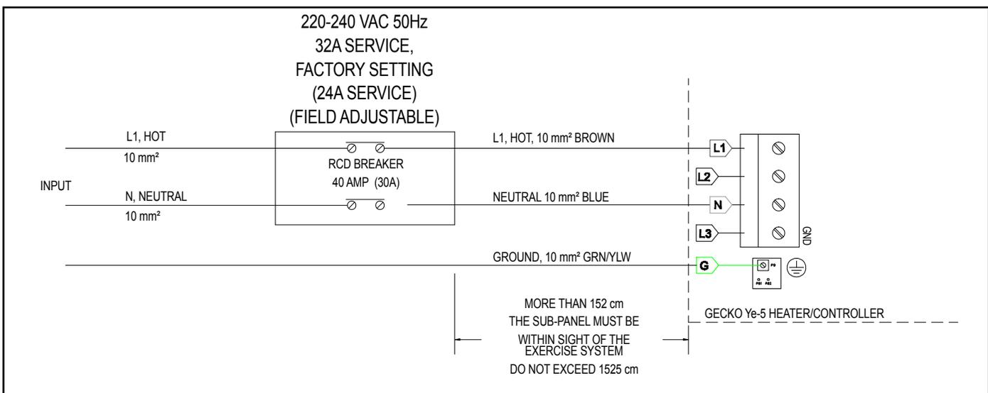
**IMPORTANT:** Using a 24A service will require a system modification, see Electrical Configuration on page 14 on how to change the system settings.
