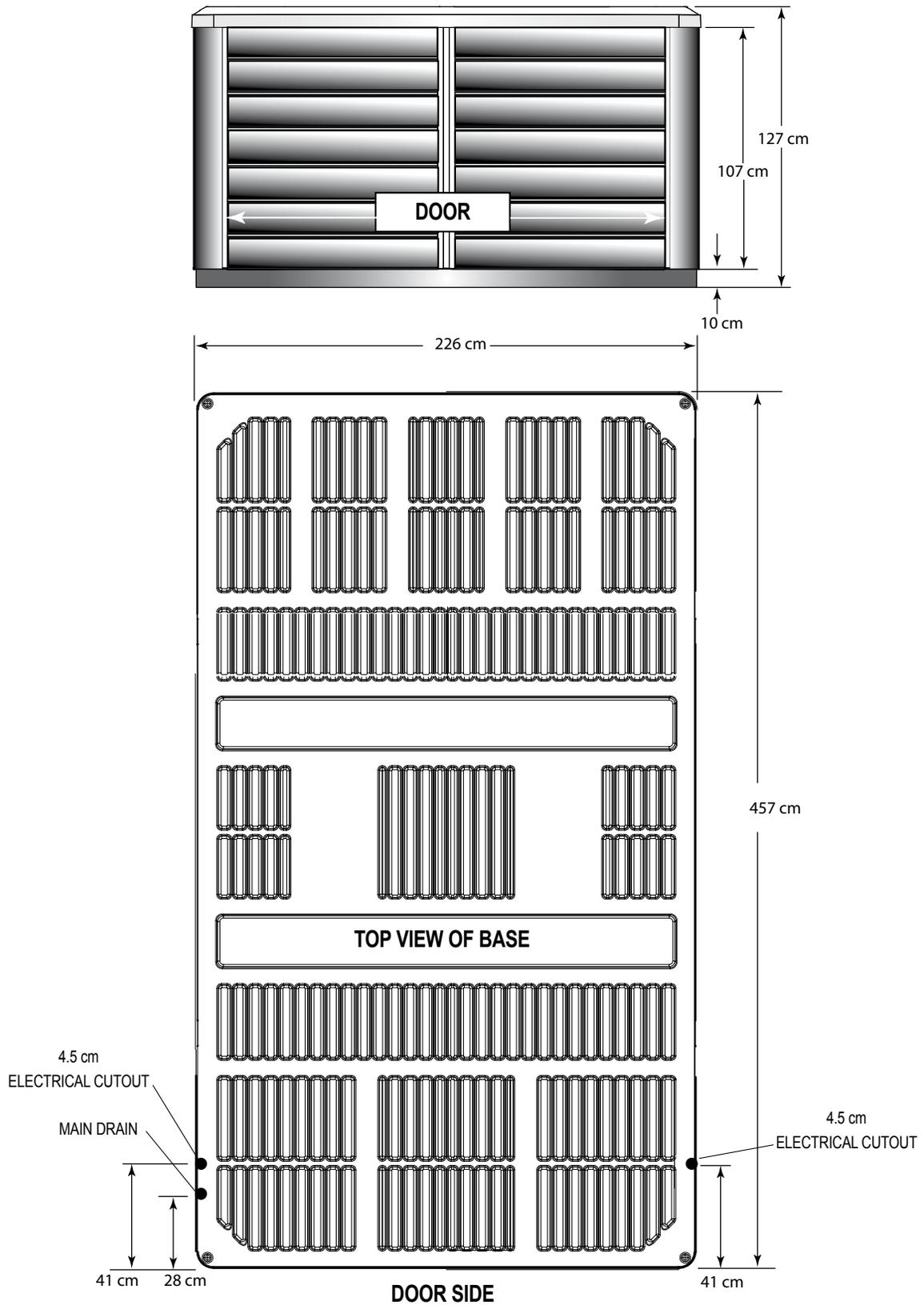
**NOTE:** ENDLESS POOLS requires that the X500 Model be installed on a minimum 15 cm (6") thick reinforced concrete pad or structurally sound deck able to support the "dead weight" found in the specification chart on the back page.
