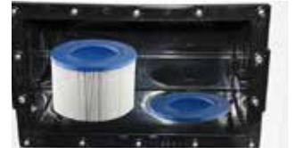
7. Repeat steps 4 & 5 to remove second filter. Always clean the filter using a filter degreaser to remove mineral and oil build-up. Simply soak the filter in the degreaser (according to the package directions), then place the filter on a clean surface and spray until clean using a garden hose. It may be necessary to rotate the filter while spraying to remove any debris lodged between the filter pleats.
