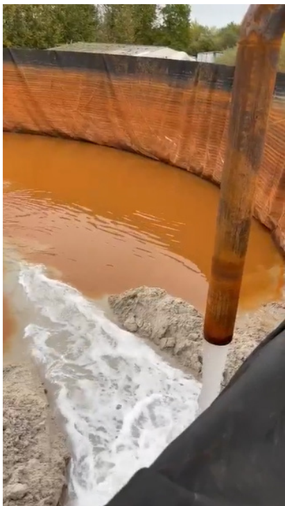
Surface test tank displays sand produced by GeoESP pump system.
