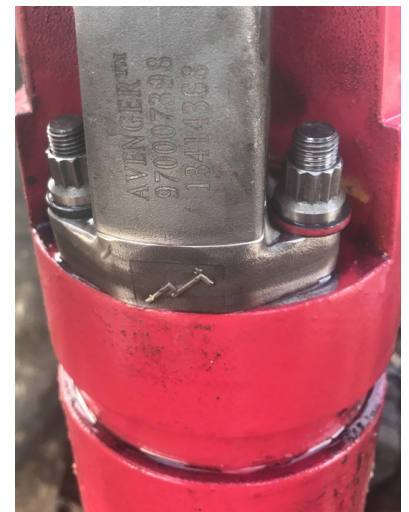
Avenger® » next generation motor lead extension.
