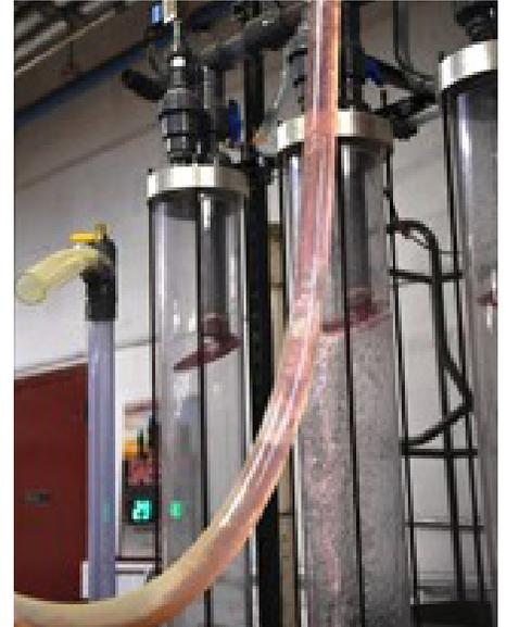
A transparent testing system enhanced the Sluggertm gas separator design.
