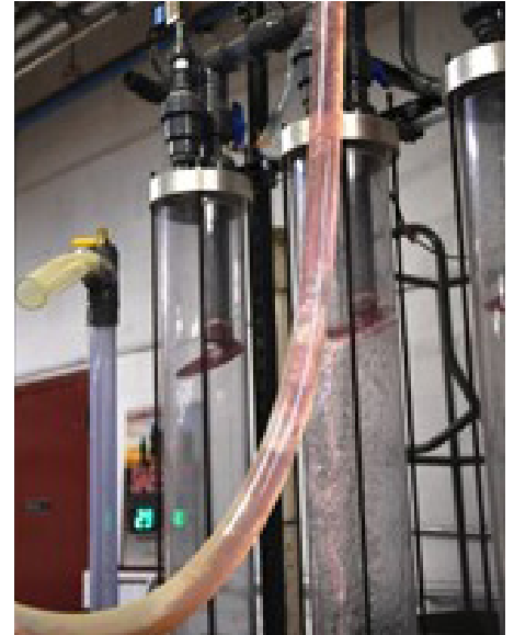
A transparent testing system enhanced the Slugger gas separator design.
