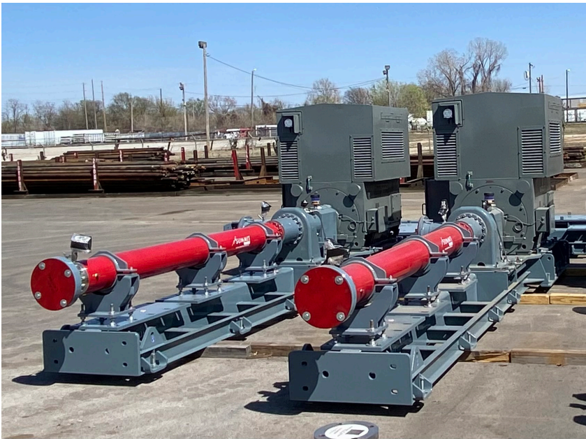
Hercules 950 series SN35000 pump systems ready to ship, prior to installation at West Texas crude oil transfer station.
