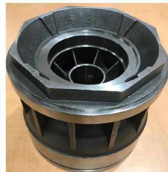
Octolock diffuser (series 675 and larger) eliminate the possibility of spinning diffusers.
