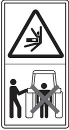
**3-pt Hitch and PTO:** Stay clear of 3-pt hitch and PTO shaft. Keep all shields in place.
