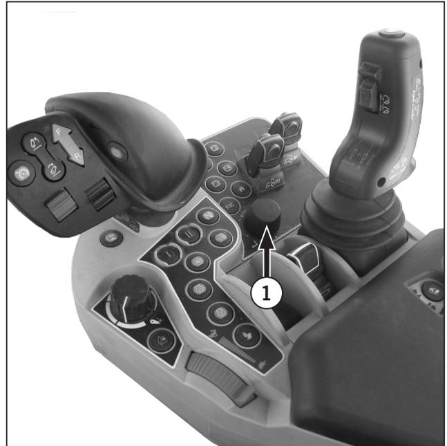
2. Press the selection dial button to make a selection. The orange selected frame turns yellow-green (1), which means the editing mode.
