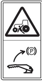
**Engage Parking Brake:** Engage parking brake before exiting the cab. See page 3-22 for parking brake operation instructions.
