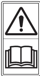
**Read Operator's Manual:** Read the operator's manual before performing maintenance or operating.
