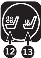
Press this switch to select either the built-in fans (12) or the heated seat cushion (13). Only 1 of these options can be turned on at a time.
