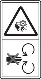
**Engine Running Warning:** Do not open while engine is running. Contact with rotating fan or belts will result in serious personal injury.
