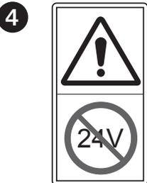
**Battery Boost Warning:** Do not boost batteries with 24 volts. Damage to electrical components can occur.
