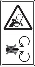
**Engine Guards:** Do not open while engine is running. Contact with belts and rotating parts will result in serious personal injury.
