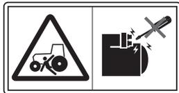
**Engine Start Warning:** Do not bypass the starter safety switch. The tractor may move suddenly and result in serious injury.
