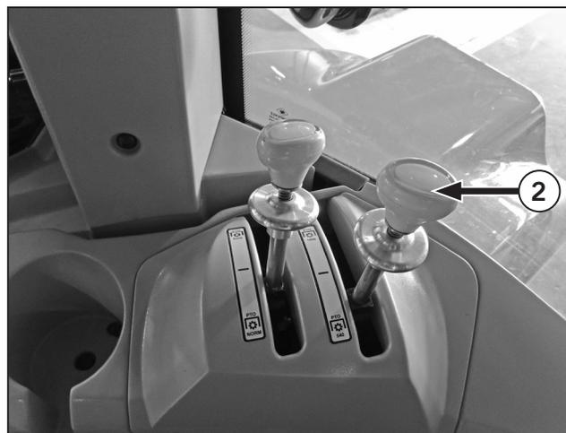
6. The PTO will shut down if a 1 000 shaft and ECO mode is selected and the PTO shaft goes above 1 150 RPM.
