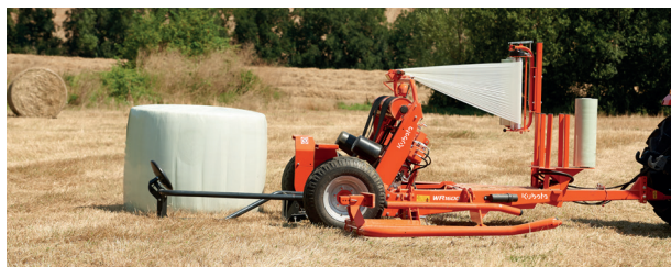
Fast and gentle on-the-move unloading with no need for a fall damper.
