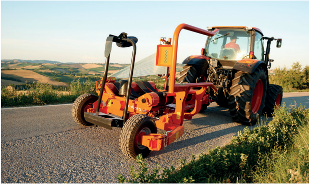
The loading arm is powered fully down to lift the wheel off the ground for easy movement from work to transport.
