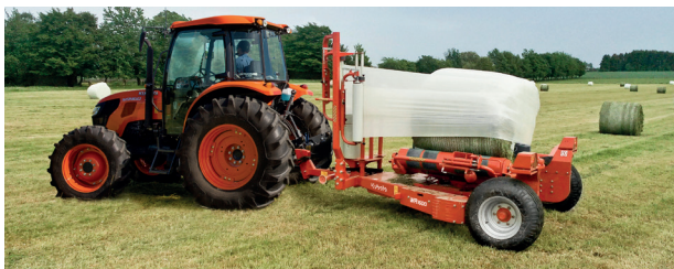
The low mounted table design allows high rotation speed.
