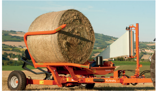
Hydraulically operated loading arm, with a low loading height, provides fast transfer of bale from arm to turntable.
