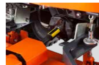
The shaft-drive PTO delivers more cutting power to the mower with fewer problems than belt drive systems.
