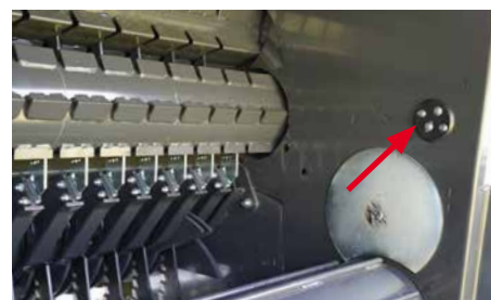
Moisture sensor located inside the bale chamber.
