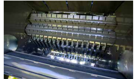
Profiled rollers provide instant bale formation and are equipped with self cleaning scrapers designed for working in all crop conditions.
