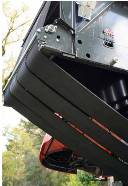
The BV6450 and BV6460 are fitted with four durable endless belts offering smooth running and low maintenance.
