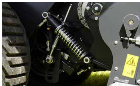
Hydraulic pick-up lift with integrated suspension system for accurate ground following.
