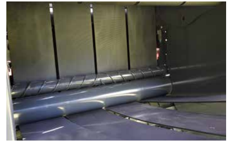
Spiral profile scrapper roller for efficient cleaning effect in all condition.
