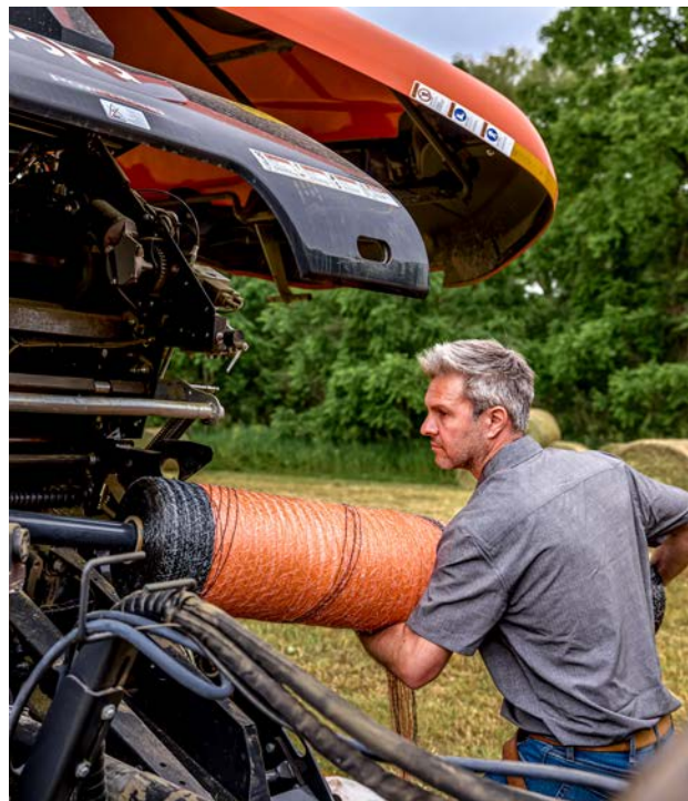
The smart net roll storage allows a comfortable horizontal loading.
