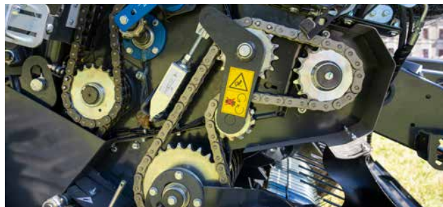
Rotor chain transmission with 1 1/4" pitch chains.
