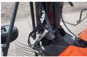
Hydraulic transport locking (optional).
