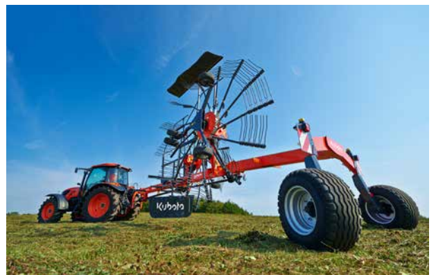
Active wheel steering for improved manoeuvrability in combination with large wheels for reduced compaction.
