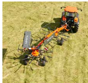
SideShift to the left - raking without driving on unranked crop.
