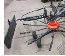
Automatic fold-able swath board with parking stand.
