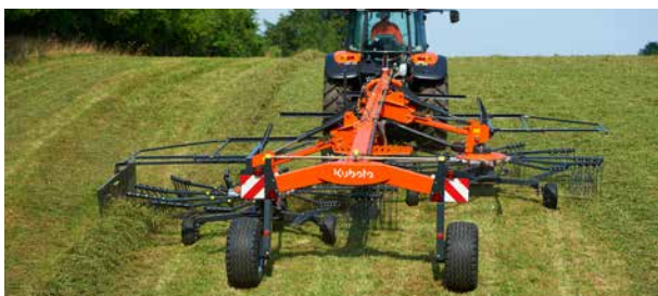
The side delivery concept allows you to collect crop from 49'2" (15.00m) into a single swath.
