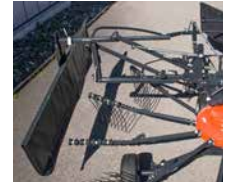
Automatic fold-able swath board with parking stand.
