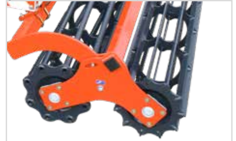
Double rouleau cage ø 15.8" (400mm) (tube/flat) - 108lbs/ft (160 kg/m)
