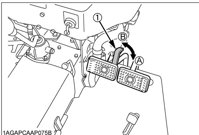
(1) Brake pedal lock (A) "LOCK" (B) "RELEASE"
