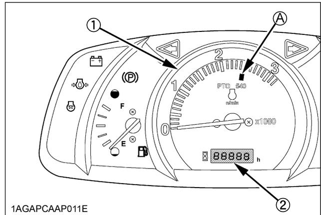
(1) Engine revolution (A) PTO : 540rpm (2) Hours used
