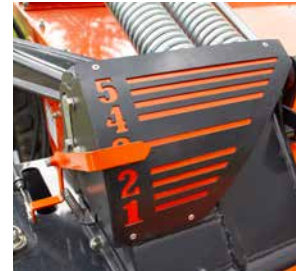
Optional hydraulic stubble height adjustment for easy setting from tractor cab.
