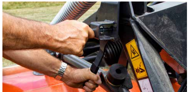
One-touch parking handle, to lock and prepare the machine for dismounting.
