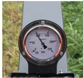
With the optional hydraulic cylinder, pressure and distance of the rollers is easily set and monitored.
