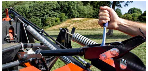
Stubble height adjustment is conveniently integrated directly into the suspension linkage. There is no need to tilt the A-frame of the tractor.
