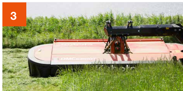
3 Mowing unit is lowered evenly onto the ground without one side touching the ground before the rest of the mower.
