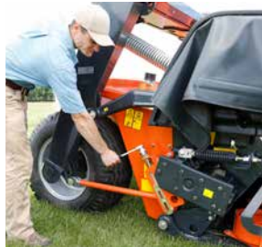
Easy adjustment of stubble height.
