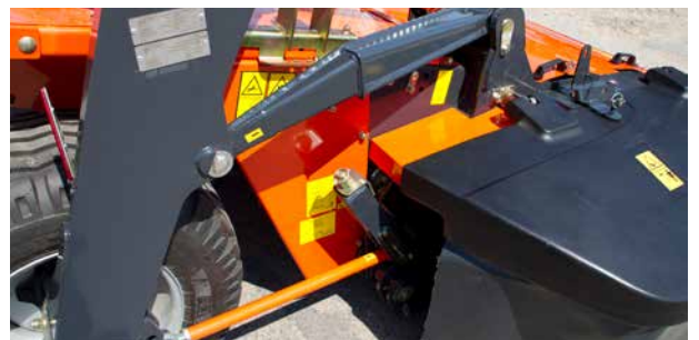
When an obstacle is encountered, the mowing section is forced backwards and the special suspension rod ensures that the mowing section is automatically lifted upwards and above the object.
