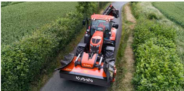
Hydraulic folding of FlexProtect guards (optional).
