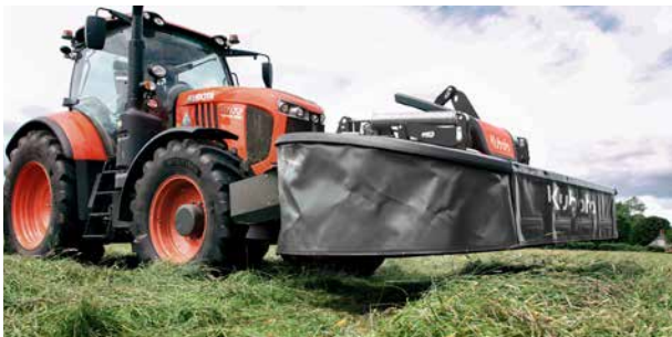
Generous ground clearance for headland turns of 17" (420mm), to pass large swaths without damaging them.
