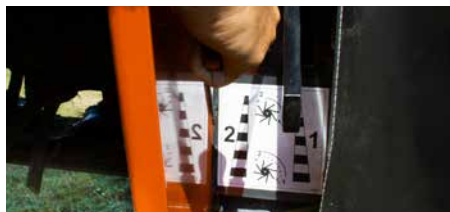
Dual adjustment of conditioner plate to customize to crop intensity.
