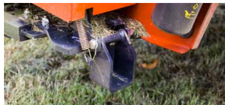
Parking foot is easily activated and keeps the mower in level position when parked.
