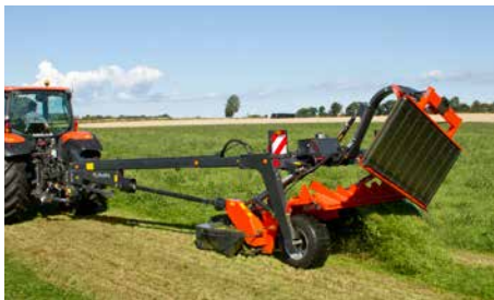
When placing the first swath, the belt is raised and hydraulically lowered for the second swath.
