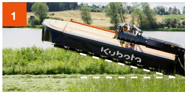
1 Minimum 1'8" (500mm) ground clearance across the complete mowing unit during headland turns. Mowing unit is raised and carrying arm tilted to a 10° angle.
