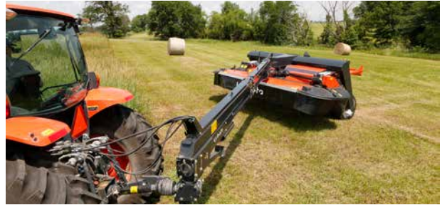
A lifting height of 20" (50cm), ensures excellent ground clearance for transport and during headland turning.
