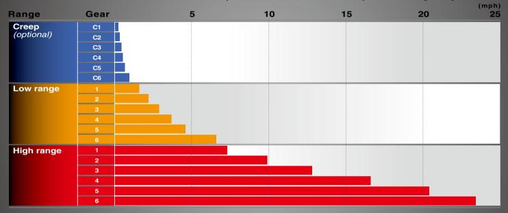
M5-091/M5-111 HDCC24 TRAVELING SPEED (F24/R24 w/ Dual Speed, 18.4-30 rear tires) @ rated engine rpm
