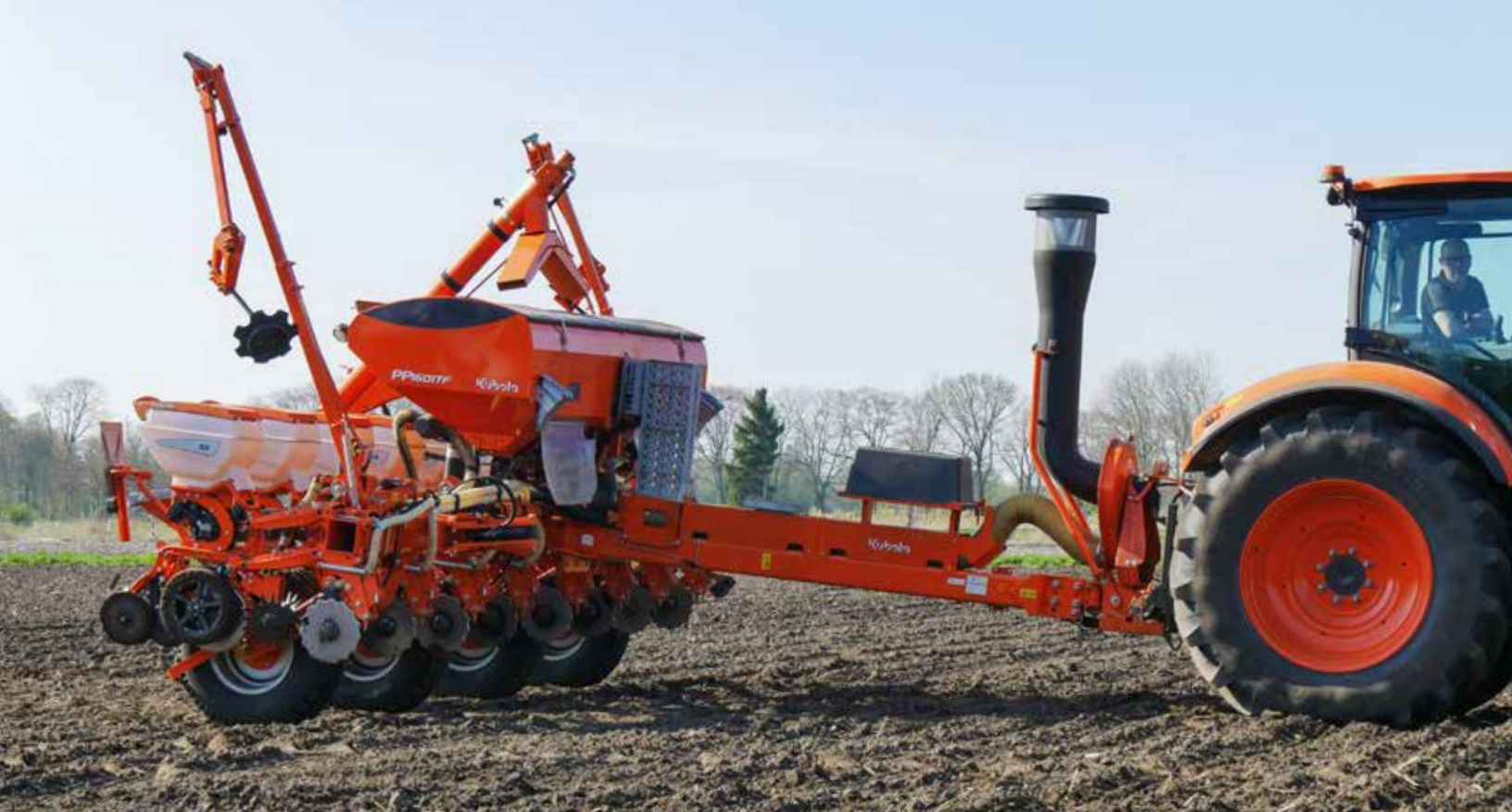
4 wheels for better balance at the headland and depth guidance in the field. PP1601TF with SX or HD-II rows.
