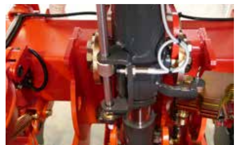
An intelligent two piece hydr. cylinder for best ground following.
