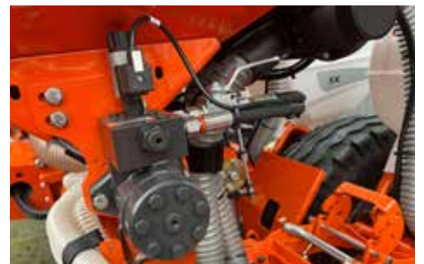
Optional electro-hydraulic drive for the fertiliser application. Fertiliser rate can be adapted even during work.
