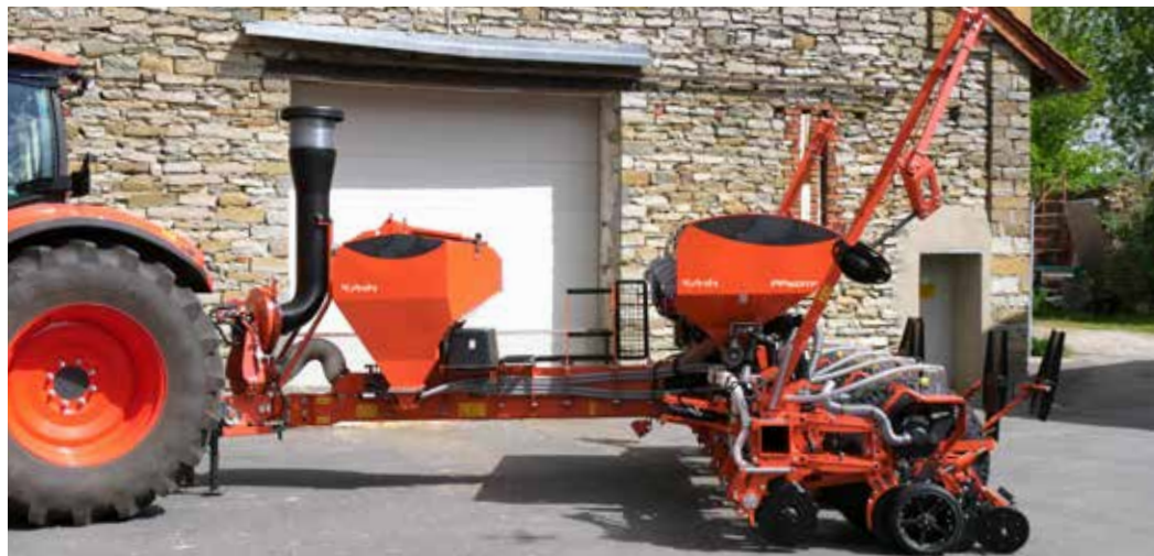
PP1601TF with SX rows and central seed hopper of 870l (25bu).
