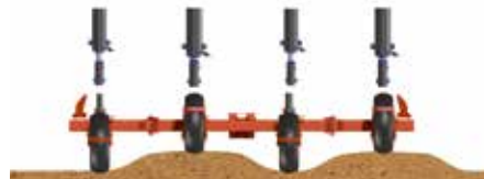
Intelligente and individual adaptation of the wheels due to the two-piece hydraulic cylinder.
