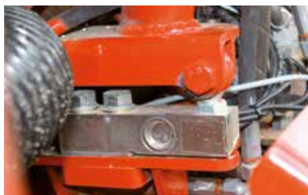
Weigh cells for the precise and controlled fertiliser application
