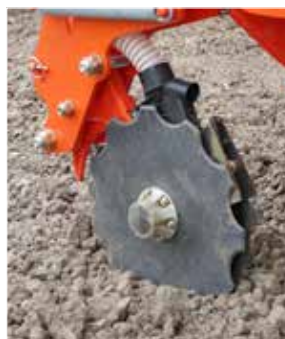
The fertilizer coultter are equipped with maintenance-free roller bearings.
