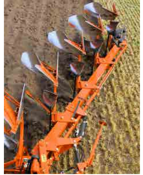
Variomat® parallel linkage.
