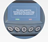
>> When operator leaves the platform, the parking brake is automatically engaged.
