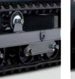
Even over undulating terrain, the bogietype under rollers contribute to more
