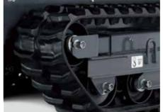
**Reinforced Rubber Crawlers** Steel reinforced cores help lengthen the life of the rubber crawlers.
