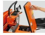
**Upper Engine Cover** The upper engine cover opens fully for easy refueling, and blocks for added protection.
