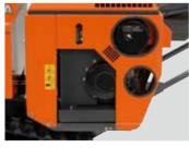
Easy Maintenance Checking and maintaining such items as the engine oil or air cleaner can be performed easily from just one side.
